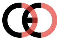
False CE Mark (too close)
