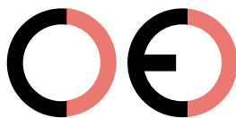
False CE Mark (too far)
